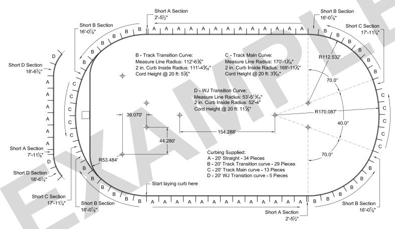
Note: Short curb sections are cut in the field from full length pieces. Lengths of short sections are approximate, actual length will need to be measured during installation prior to cutting the short sections. Notched ends are not required on short sections. To allow for curb expansion on hot days, 1/16" to 1/8" gaps should be left between each curb section. The temperature of the curb during installation should be taken into account when setting the gaps.
