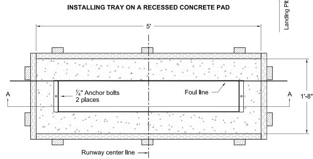
When positioning tray on base concrete, insure tray sits flat and does not warp when anchored in place. The tray lid should not rock if tray is properly installed. When finishing runway subsurface around the sides of the tray, insure the procedure does not deform the tray sides inward.
