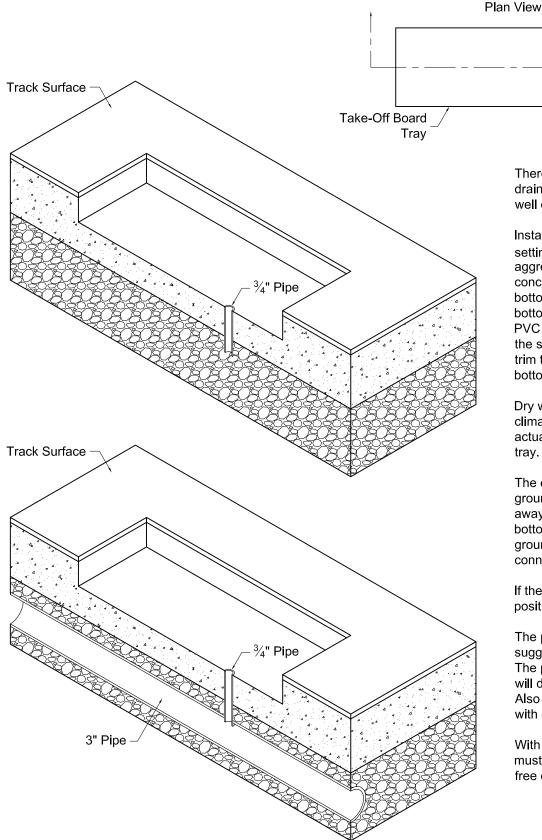
There are basically two options for draining the take-off board tray; a dry well or an under ground drainage pipe.
