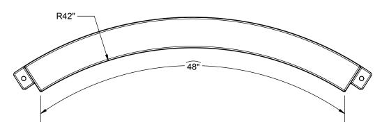
The 364 Cast Aluminum Toeboard is designed to be used on a level throwing surface with a Gill 373 Steel Shot Circle or the 372 Aluminum Shot Circle. The 364 toeboard can also be mounted over a 2" wide painted circle.
